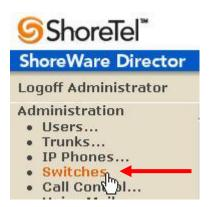
This action brings up the "Switches" screen. From the "Switches" screen simply select the name of the switch to configure. The "Edit ShoreGear ...Switch" screen will be displayed. Within the "Edit ShoreGear ...Switch" screen, select the desired number of SIP Trunks from the ports available.
